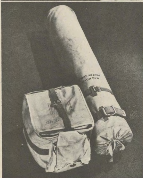
Emergency radio. One case contains the radio, and the other contains accessories for operating it, including the following items: balloon and kit for raising antenna, hydrogen generators for inflating balloon, signal lamp, extra roll of antenna wire, and an instruction book. A parachute for dropping the radio to survivors is attached to the accessory case.
