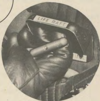
There are two raft release handles. Pull both handles to release and inflate both rafts.
