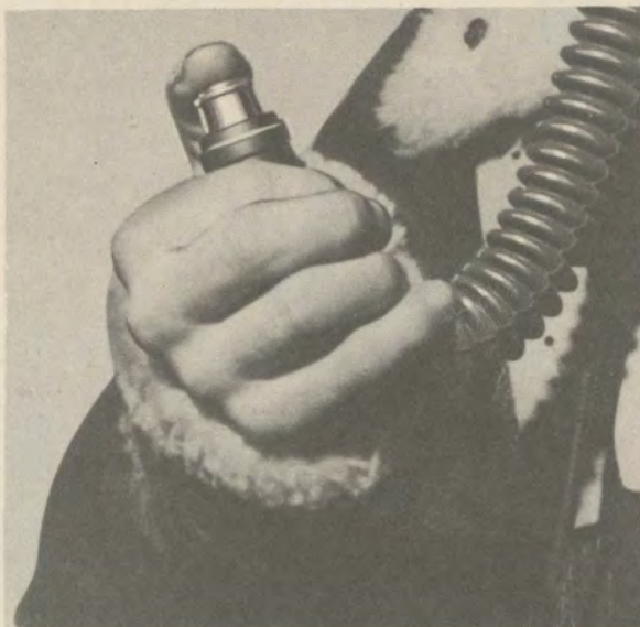
Gentle suction test for mask fit.
