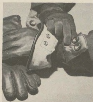
Turn up rheostat to see that suit heats; then turn it back off.
