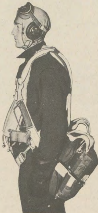
Seat-type parachute with individual type B-4 emergency kit.
