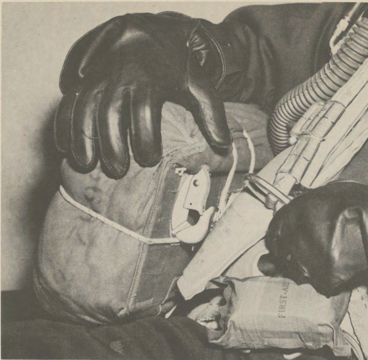
Attach chest-type chute like this, ripcord on the right-hand side.
